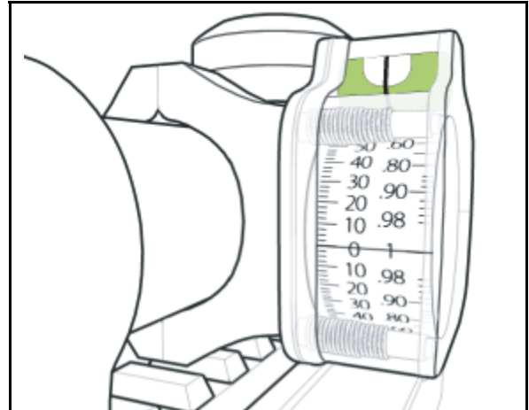
Left-handed shooter, bubble level up Mounted on right side of the optic for left-handed shooters, with bubble level on the top
