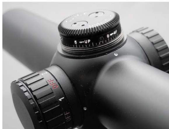
Figures 1-3: Slipping the elevation and adjustment knobs’ scales to “0” will provide a definitive index point to return to in the event you ever adjust them off zero.
