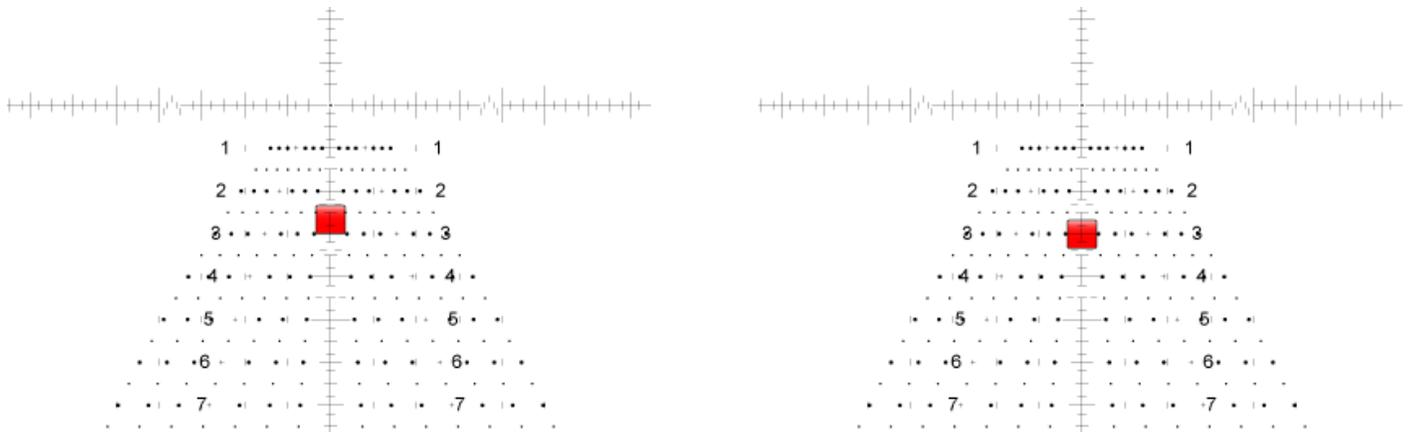
**Figure 14:** (LEFT) The reticle image at left depicts a 12-inch target best bracketed by the Speed Shooting Drop Marker on the 3-mil drop line. (RIGHT) At right, the target is then vertically centered directly behind the 3-mil drop line.
