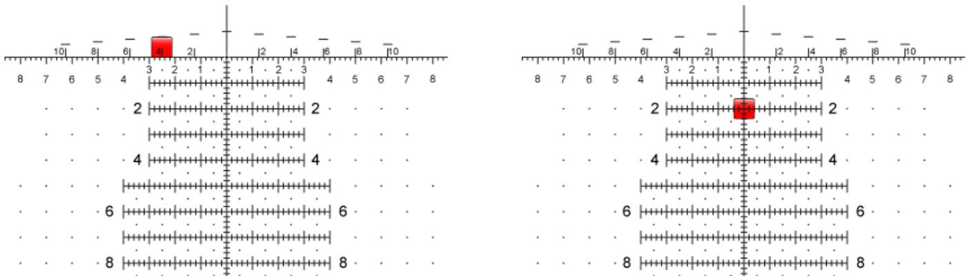
**Figures 6:** (LEFT) The reticle image at left depicts a 12-inch target bracketed between the main horizontal stadia and the line above the "4" moving target hold. (RIGHT) At right, after dividing the "4" in half, an elevation hold of "2" is used to engage the target's center mass.
