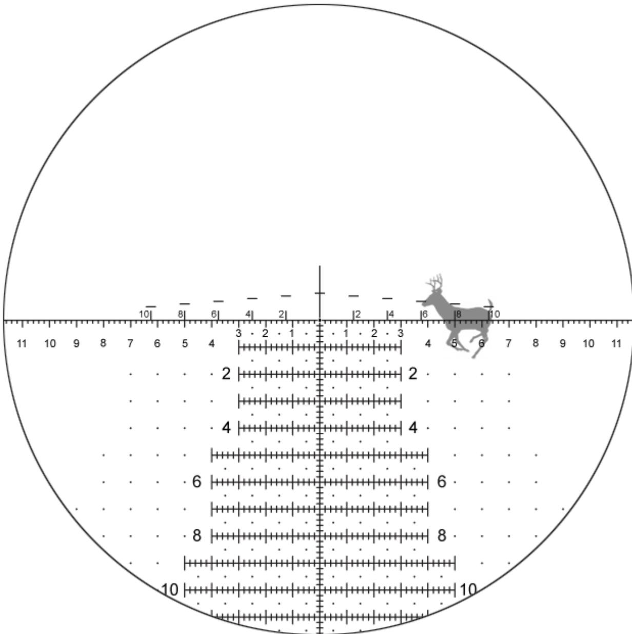
**Figure 5:** The Accuracy 1<sup>st</sup> Speed Shooting Formula allows use of the numbers along the horizontal stadia to rapidly acquire moving targets. This example shows a hold for a target running at approximately 8 mph, from right to left.
