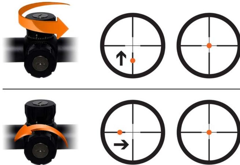
**Figure 1:** Rotating the elevation turret counter-clockwise will move the POI up in the field of view (top). Rotating the windage turret counter-clockwise will move the POI right in the field of view (bottom).
