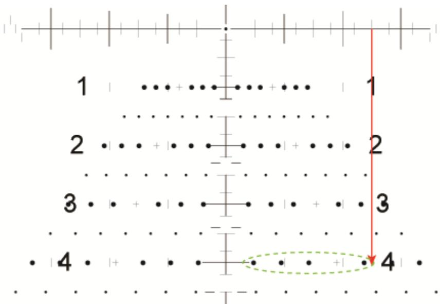
**Figure 10:** The Ballistic Solver method for determining wind marker values is illustrated for a 20 mph wind with a 2.5 mil wind hold and 4 mil drop hold. To determine TReMoR2 wind values, we divide the wind speed (20 mph) by the number of TReMoR2 wind markers (5, circled in green) which occur on the 4-mil drop line before the 2.5-mil wind hold:  $20 / 5 = 4$ . Hence, 4 is the TReMoR2 wind value.
