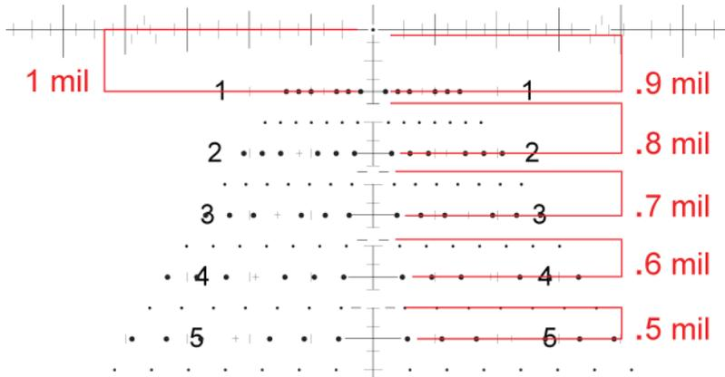
**Figure 13:** Speed Shooting Drop Markers are embedded directly into the TReMoR2's main vertical stadia from drop lines 1 - 5, providing a visual system for rapid drop adjustments for targets out to 600 meters. As shown in red, marker heights decrease by 0.1 mils from one Speed Shooting Drop Marker down to the next.
