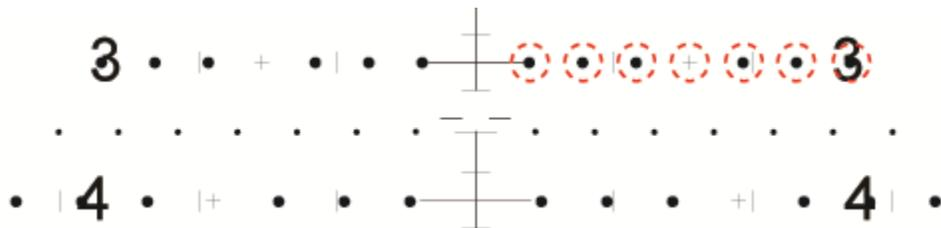
**Figure 8:** Seven wind markers occur on each side of the reticle along drop lines 1 – 9, circled in red above. Similar but smaller wind markers occur along half-mil drop lines, visible here at the 3.5-mil drop line. Crosses designate 4<sup>th</sup> markers, making counting faster and easier, shown here on the 3 and 4-mil drop lines.
