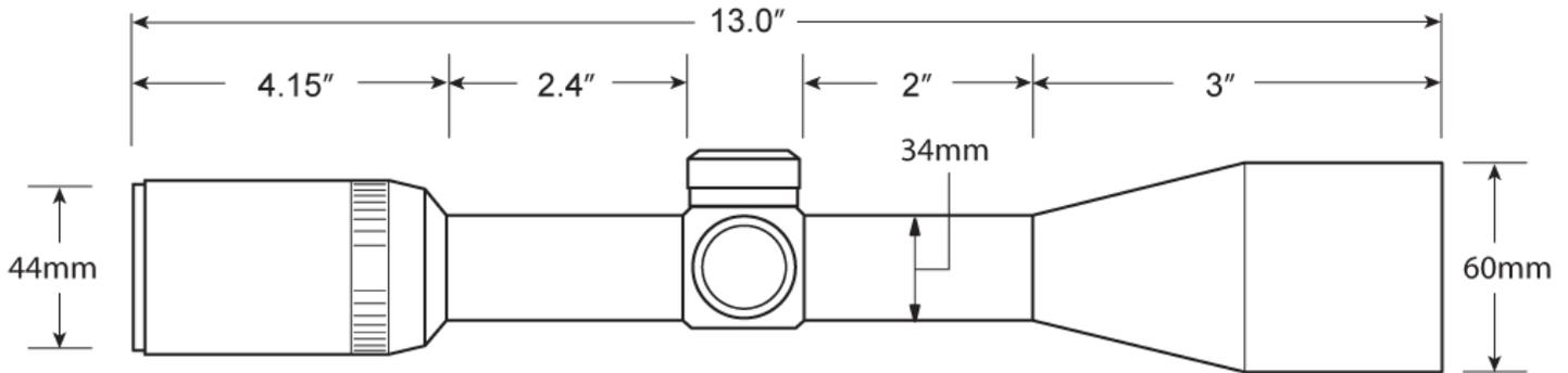
Figure 15: HDMR scope technical drawing with specs.
