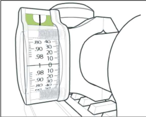
Right-handed shooter, bubble level up Mounted on left side of the optic for right-handed shooters, with bubble level on the top
